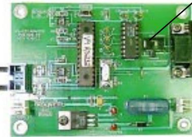
null modem switch allows you to reverse pins 2 & 3
